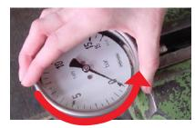
4. Turn the ring by hand and remove it straight upwards without touching the inner parts.
