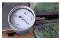
1. Fasten the pressure gauge adequately (e.g. in a vice).
