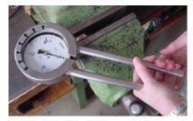
Place the clamping ring on the device and clamp it with one hand.
