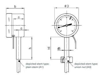
Compared to the basic models, the following dimensional changes or additions result for thermometers with reed contact:
