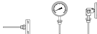
TBiSch...rm TBiSch... TBiGelCh... with bayonet ring TBiSchG...rm TBiSchG... TBiGelChG... with crimped-on ring Figures show bayonet ring cases
