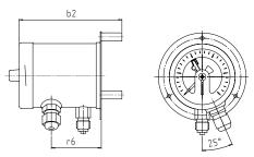
Case configuration Rh is supplied with 3 loose mounting spacers.
